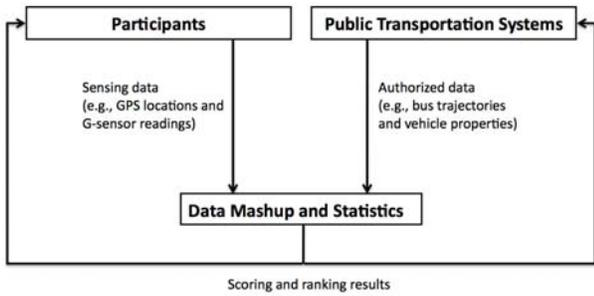
**Figure 1: The architecture of the CMS system**
