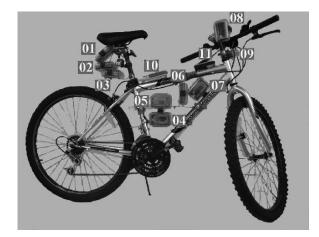
Fig. 3. Physical implementation of the BikeNet system. Numbered sensors installed on the bicycle map to the sensor types labeled in the logical BAN representation in Figure 2.
