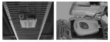
(c) A BikeNet static SAP is a WiFi AP with an (d) Waterproof OtterBox. Wires are fed through Invent inserted in the USB port. drilled holes that are then filled with silicone sealant. Wires have crimped connectors for easy
