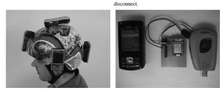
(e) Ground-truth video/sound/photo helmet with (f) BikeNet mobile SAP implementation. The four N80s and GPS receiver, only for use in de- Nokia N80 Bluetooth radio associates with a bugging our system and validating our inference custom-built Bluetooth/802.15.4 gateway. techniques.
