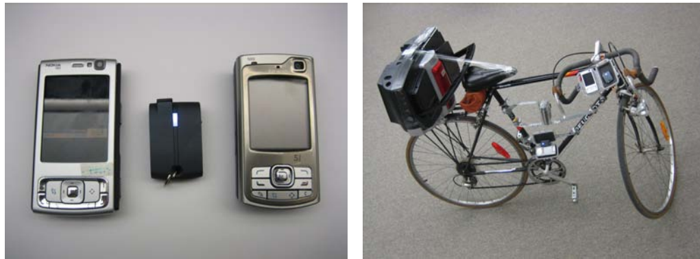
(a) From left to right: N95, GPS dongle, N80. (b) Boombox bike used as mobile sound target.
