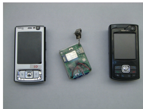
Fig. 2. The BluCel device provides a 3D accelerometer that can be connected to the mobile phone (e.g., Nokia N95 or N80) via Bluetooth.
