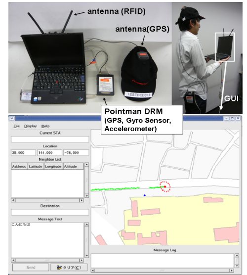
Fig. 5: P2P-based localization system.
