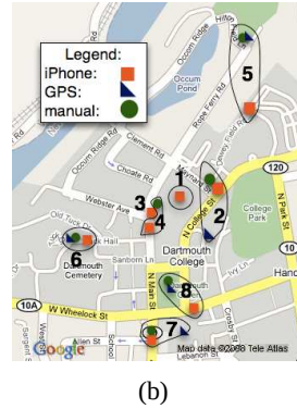
Fig. 2: (a) Battery duration with and without CenceMe running while the iPhone screen saver is set to off. - Localization accuracy for eight different locations in the Dartmouth campus of (b) the old iPhone (no GPS), and (c) the iPhone 3G (with GPS).
